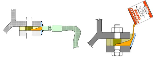
The outer metal dam can be installed at an angle.
